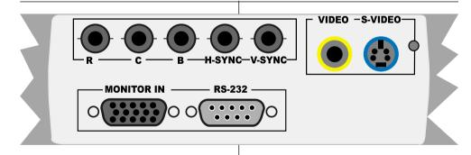
Figure 6 Connecting to video sources
